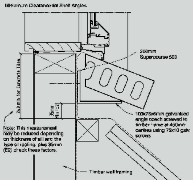
A minimum clear distance of 240 mm should be allowed for between the roof and the base of the window. This is to allow for adequate fixing of the masonry and to accommodate the window sill.
