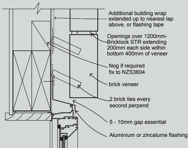
**Fig F. Head Flashing**
