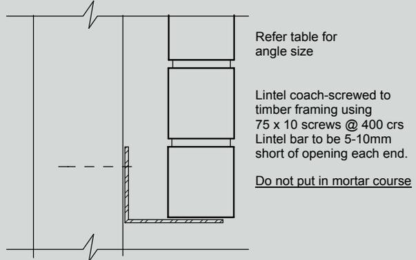
**Fig C. Steel-less Lintel- Standard Stretcher**
