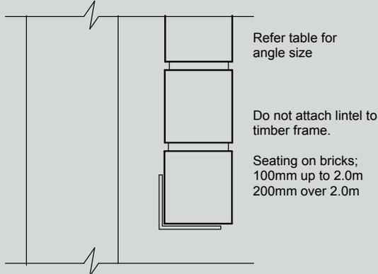
**Fig B. Lintel- Fixed to framing**
