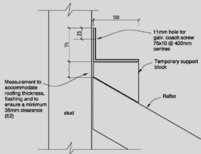
**IMPORTANT:** Ensure that where 'Shelf Angles' are to be fixed, there is no possibility of the coach-screw penetrating electrical cables, or water pipes.
